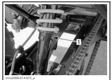
**REAR SUSPENSION** 1. Preload cam
